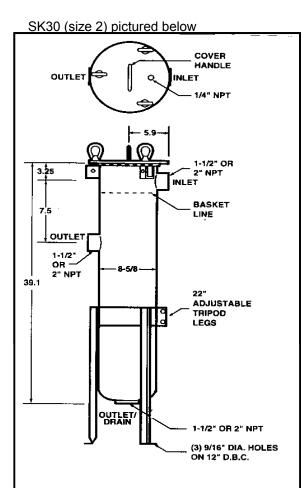
\*Based on housing only. Fluid viscosity, filter bag used, and expected dirt loading should be considered when sizing a filter.
