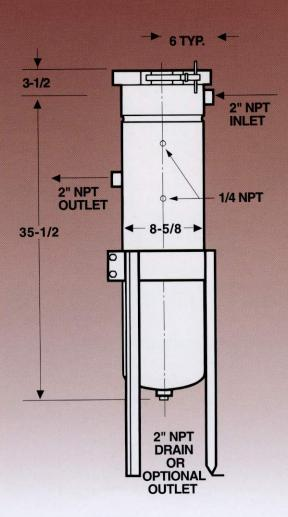
The Knight KLC is our low cost, high capacity filter bag vessel. The unique design of KLC offers you the option of a side or bottom outlet. There is a 2 inch outlet on the side, with a 2 inch plugged drain at the bottom of the vessel. The outlet can be changed to the bottom by simply moving the plug from the drain to the side outlet.
